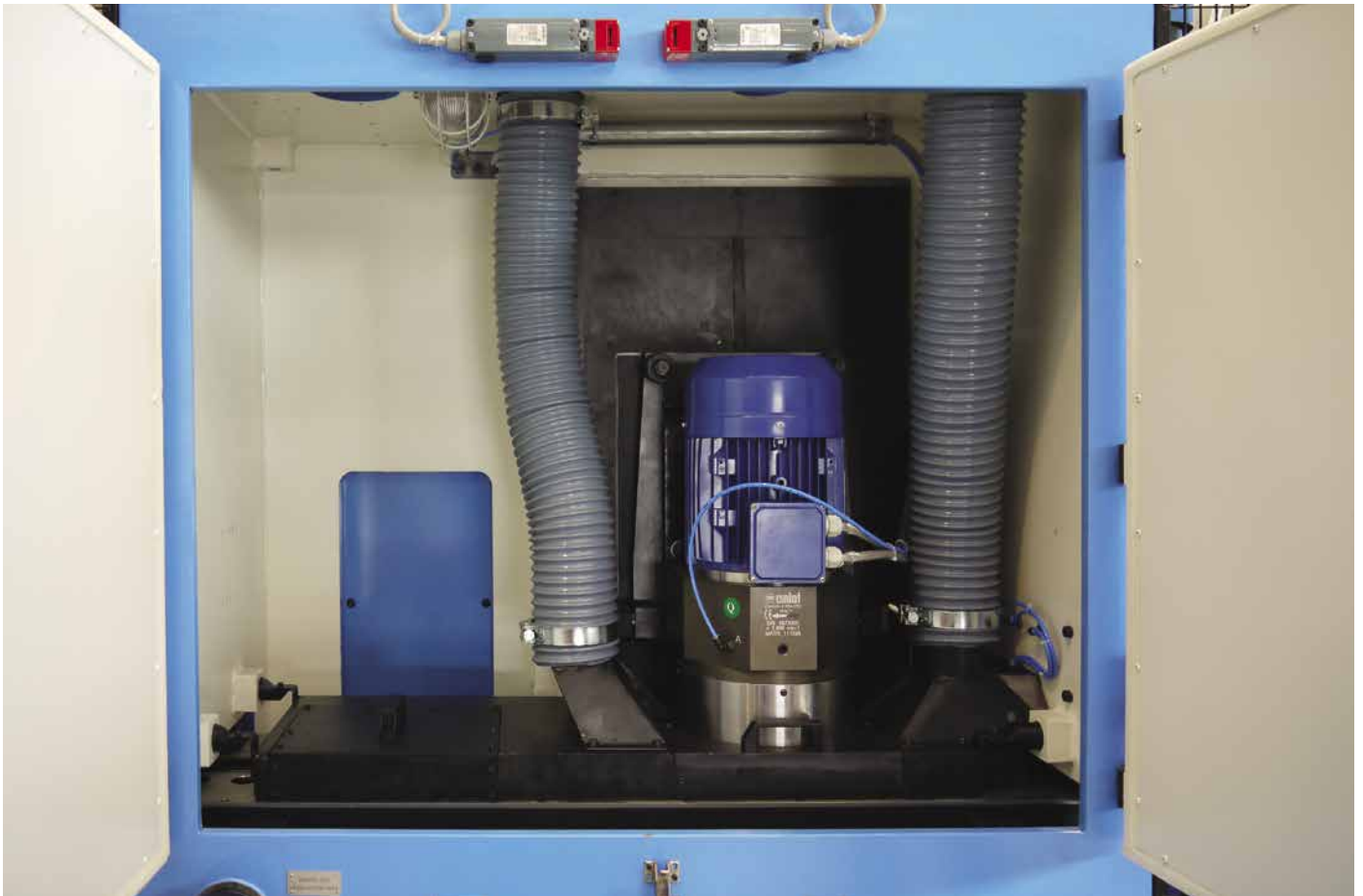
Machine inside – Grinding head and cutting arrangement
