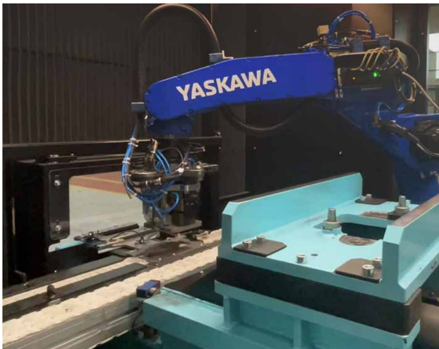
Gripper that pick up the pad
